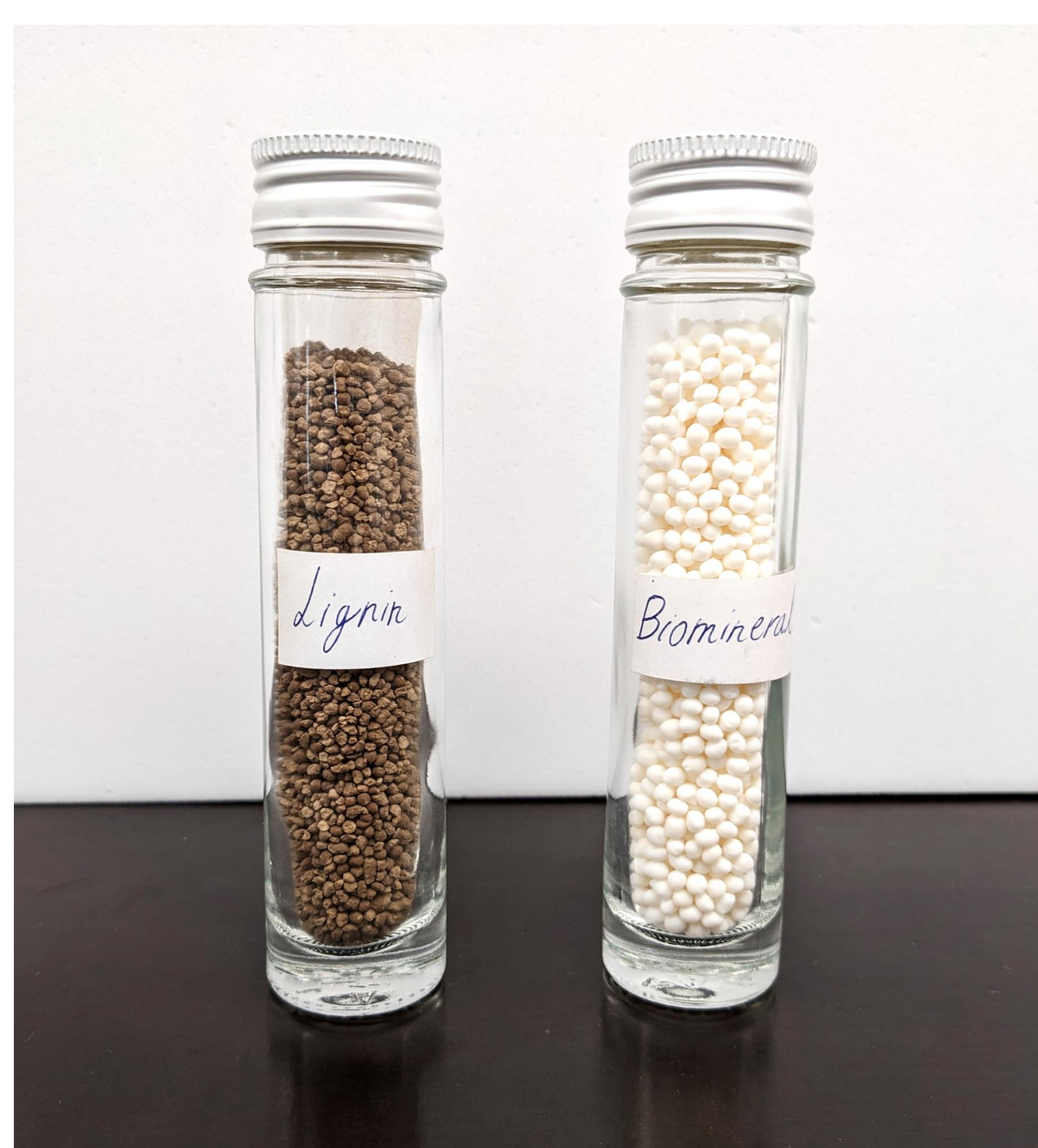
Fig. 2. Bioaerogel based on lignin (left) and silica biomineral aerogel (right)
